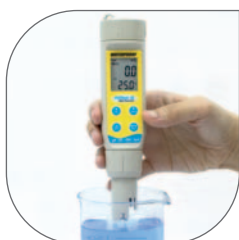
Step 1: Immerse tester sensor in solution
