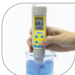
Step 3: Press "MODE ENT" to toggle to the next parameter
