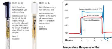
Temperature Response of the Orion ROSS Electrode Orion 81-02 vs. Conventional Electrode
